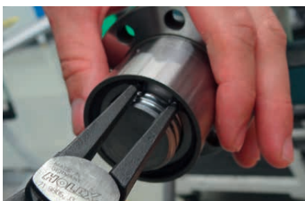
Fig. 4.9 Removing the circlip
