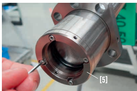
Fig. 4.16 Unscrewing the wiper housing
